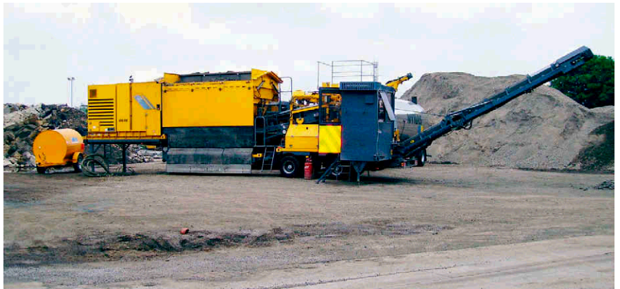
Tar bound asphalt arisings can be recycled back into the road safely with the Foambase process
