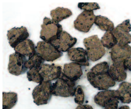
Stripping and boiling tests on stone coated with conventional bitumen showed 5% coverage remaining (left), while only 5% of Shell's new binder was lost from the same type of stone and tests
