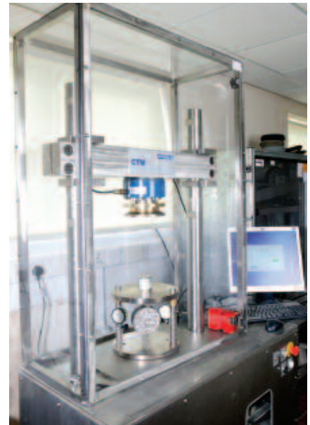
Nynas has the equipment needed for developing EME2 mixes – including a Duriez machine
