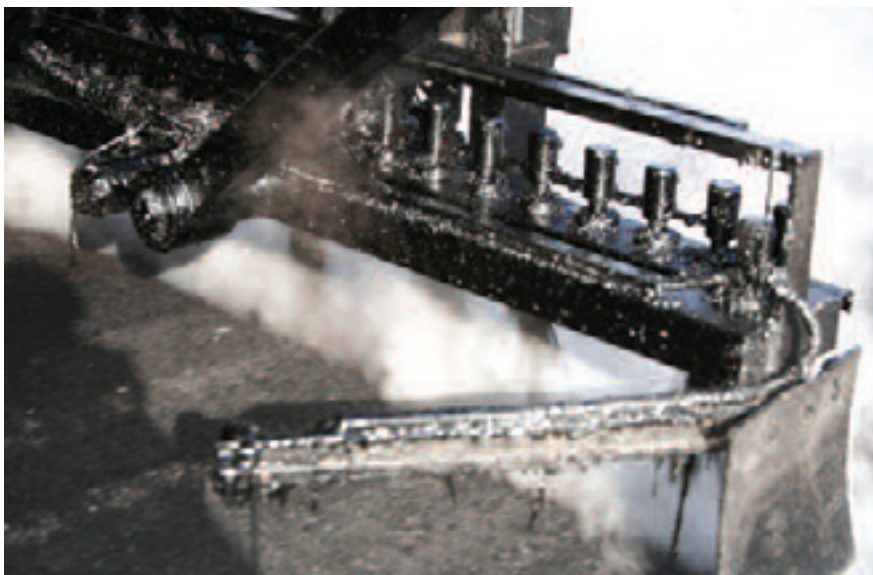
Nybreak mixed in the spray tanker jets can reduce breaking time by up to two thirds
