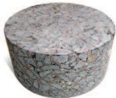
Flexicrete road surface sample before being soaked in petrol
