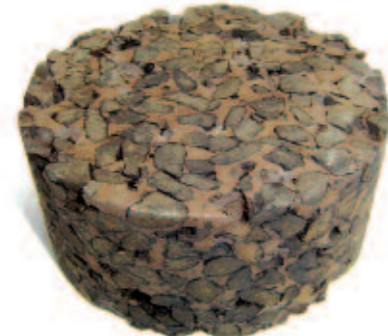
Flexicrete road surface sample that has been soaked in petrol for 15 days
