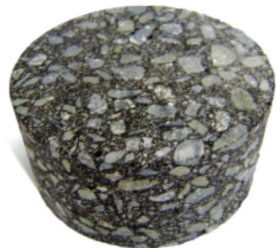
Normal road surfacing sample before being soaked in petrol
