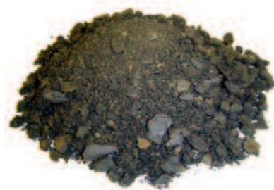
Normal road surfacing sample that has been soaked in petrol for 15 days
