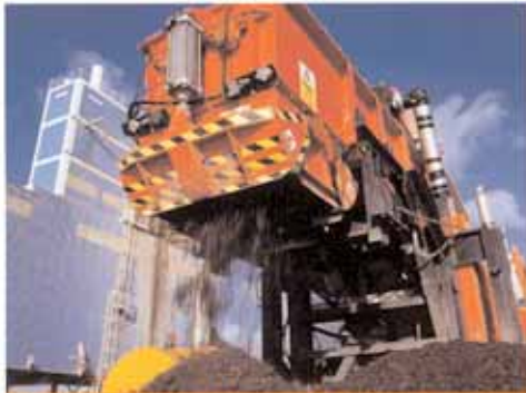
RMC's new mobile cold mix asphalt plant allows asphalt to be recycled on site using foamed bitumen technology.
