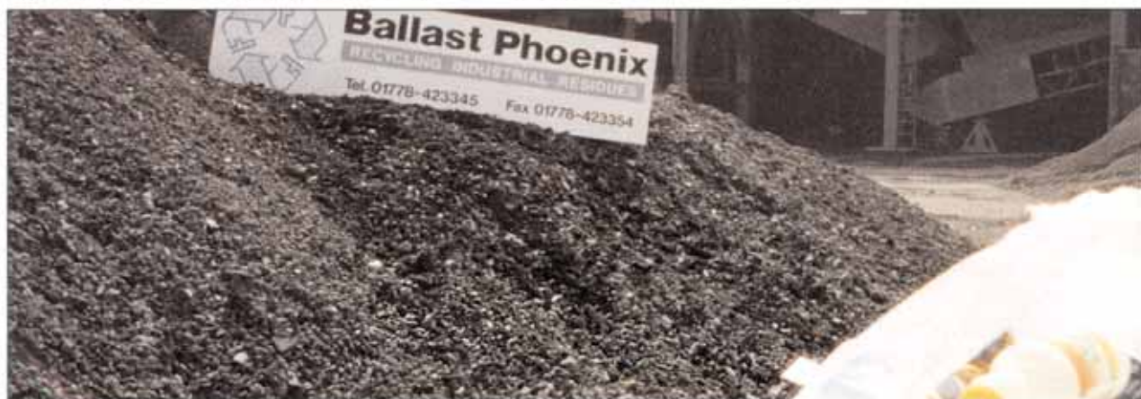
Waste from Edmonton incinerator is used in one of the most successful versions of Foamix.
