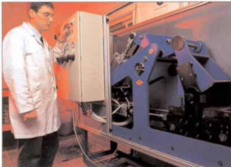
Slabs of Viatex are prepared using a segmental roller compactor at RMC's NAMAS accredited laboratory
