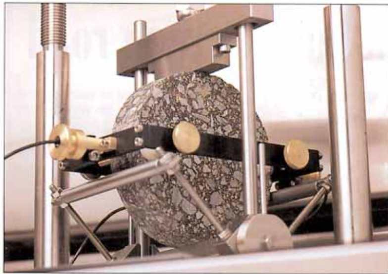
left: Strain and fatigue performance values are quantified using a CRT-NU-5 asphalt tester.
