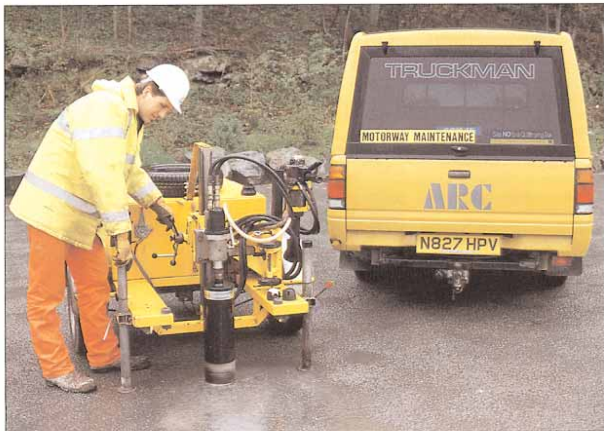
Taking proper cores is a vital part of laboratory analysis of material performance
